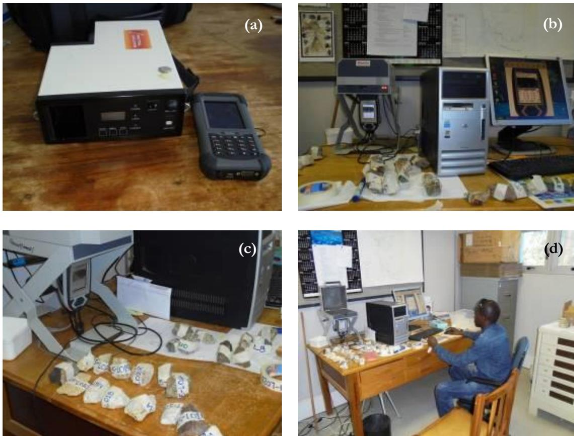
Figure 3. (a) The spectral evolution device (b) the Niton XL 3t Gold+ XRF device (c) a display of rock samples in the laboratory for XRF measurements (d) XRF measurement setup at the Geological Survey of Namibia (Geochemical Laboratory).
