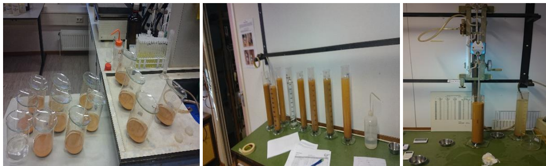
Figure 4.6: Soil texture determination in ITC Geoscience Laboratory using the pipette method
