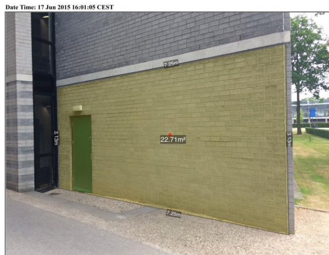
Figure 3.4: Sample measurement made using spike laser device
