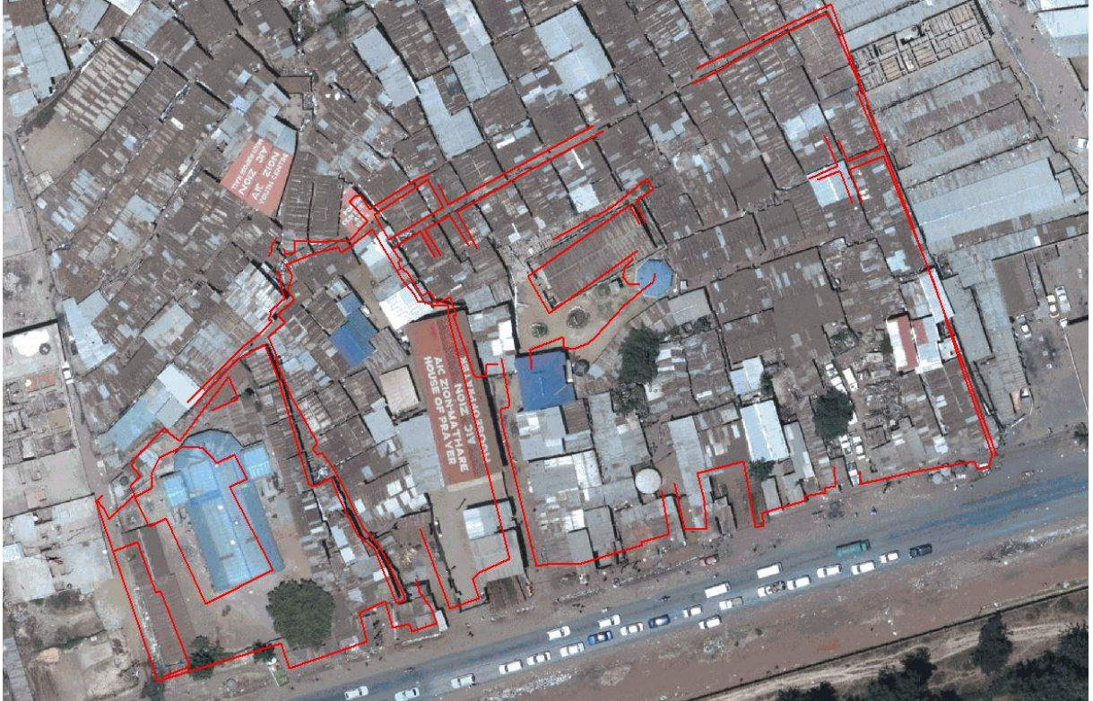
Figure 4.20: 2D outline of the slum overlaid on orthophoto
