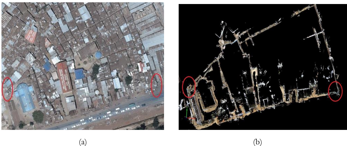
Figure 4.14: Corresponding points in orthophoto and point cloud
