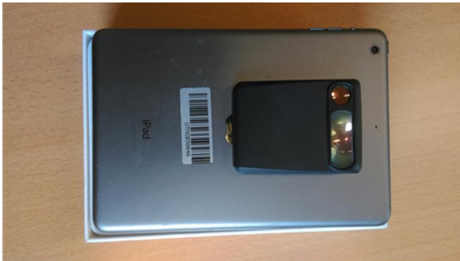
Figure 3.2: Spike laser device mounted on an iPad®
