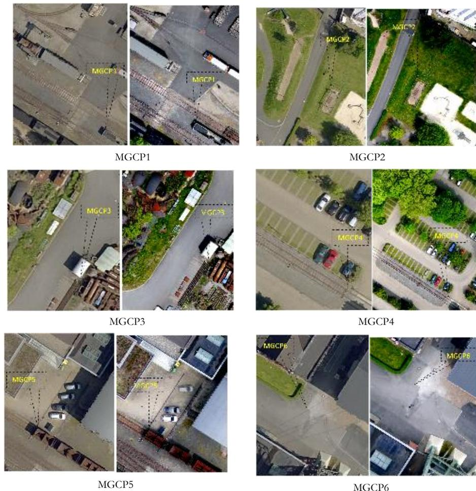
**Figure 3-6:** Control points selection from aerial orthophoto on left side and UAV orthophoto on right side.
