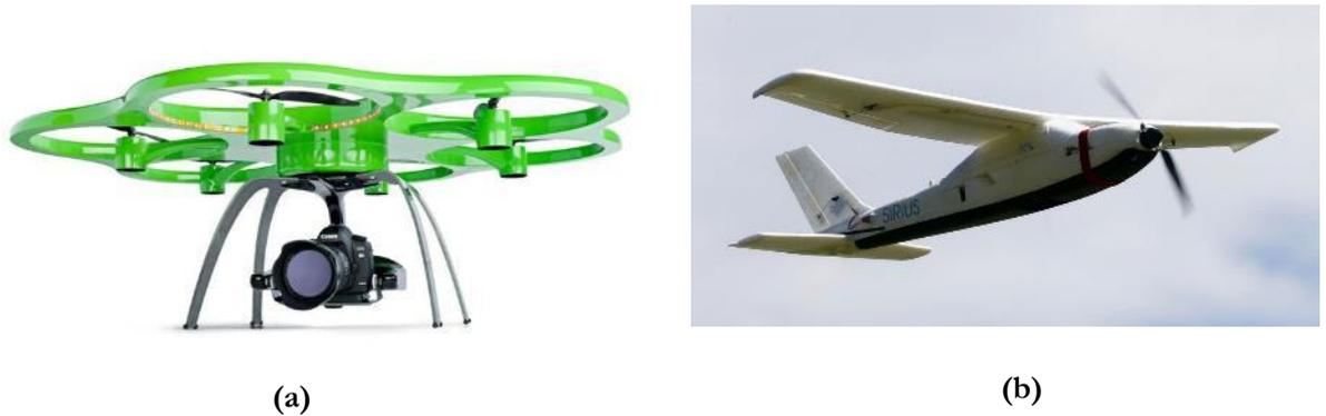
**Figure 2-1:** Example of UAV platforms, (a) Aibot X6 Hexacopter Rotary Wing; (b) MAVinci SIRISIUS Pro Fix Wing
