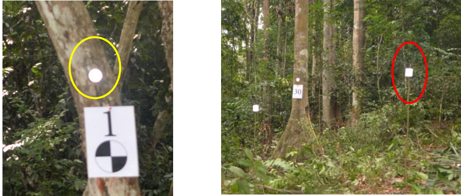
Figure 10: Circular (left) and cylindrical (right) retro-reflector used as a tie point.
