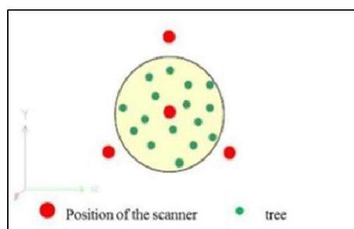
Figure 9: TLS scan positions used for the study. Source: (Bienert et al., 2006).
