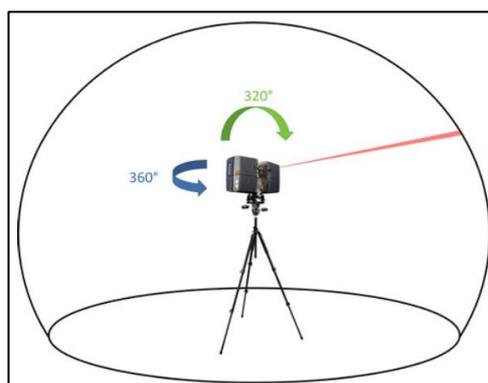
Figure 4: Operating principle of a terrestrial LIDAR. Source: (Dassot et al., 2011).
