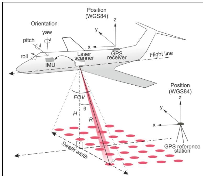
Figure 2: Typical operation of an Airborne LIDAR scanning system. Source: (Gallay, 2013).
