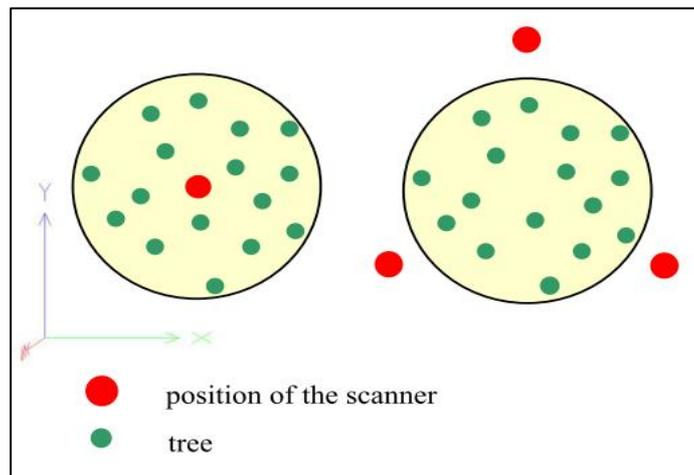
Figure 5: Single and multiple scanning methods. Source: (Bienert et al., 2006).
