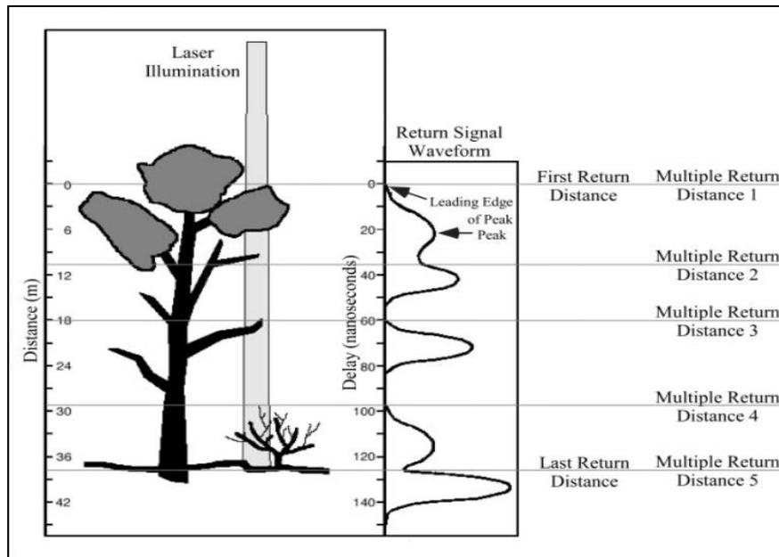
Figure 3: Airborne LIDAR discrete-return and full waveform returning pulse signals. Source: (Lefsky et al., 2002).
