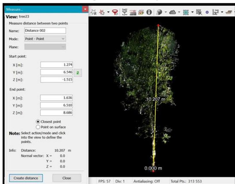
Figure 15: Tree height measurement (Plot 3, tree number 23).
