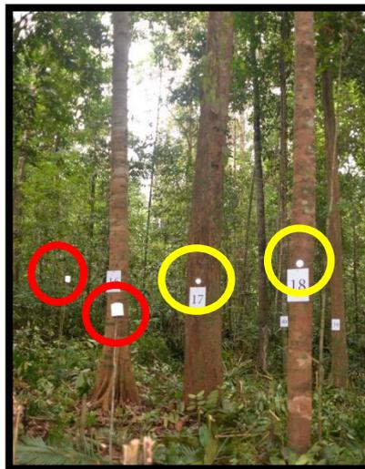
Figure 11: Setting of circular (yellow color) and cylindrical (red color) reflectors in sample plots.
