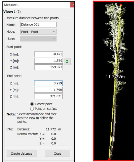
Figure 13. Individual tree height measured from extracted point clouds found in the upper and lower part. Which means the difference between the two-point cloud gives the height of the tree.
