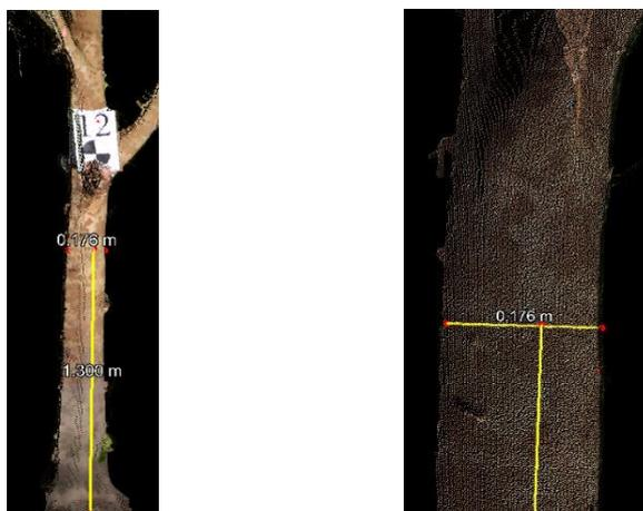
Figure 12. Individual tree DBH measured from manually extracted point clouds using measuring tools in RiSCAN PRO software.
