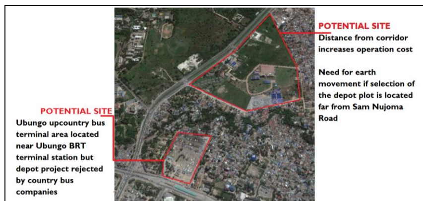
Figure 51 Potential depot sites to opposite DSM University Source: Researcher, 2016 , Google earth imagery date 2016
