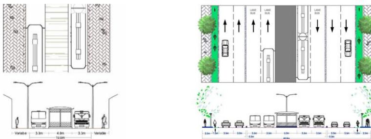
Figure 44 Constricted 10m width to optimal BRT 40m width BRT median station set ups
