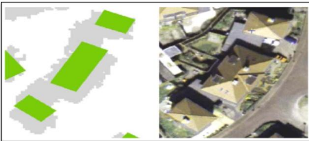
Figure 1-2: Detected mapping error, operator mapped three separate buildings the LiDAR data shows that buildings were connected by lower part with flat roofs (Source: Vosselman et al. 2005).
