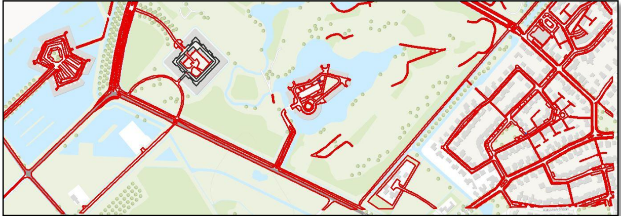
Figure 4-15: Road polygon overlaid on the reference data. Verified road class(red), change(grey) and unknown(blue).
