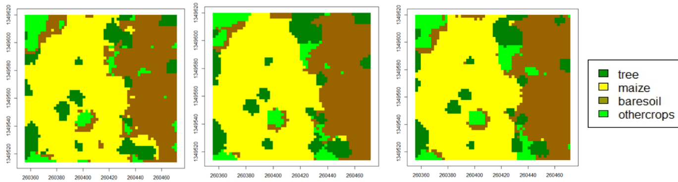
Figure 31. MPS classification results with different number of simulations, from left to right there are three different MPS classification results with 10, 20 and 30 simulations.
