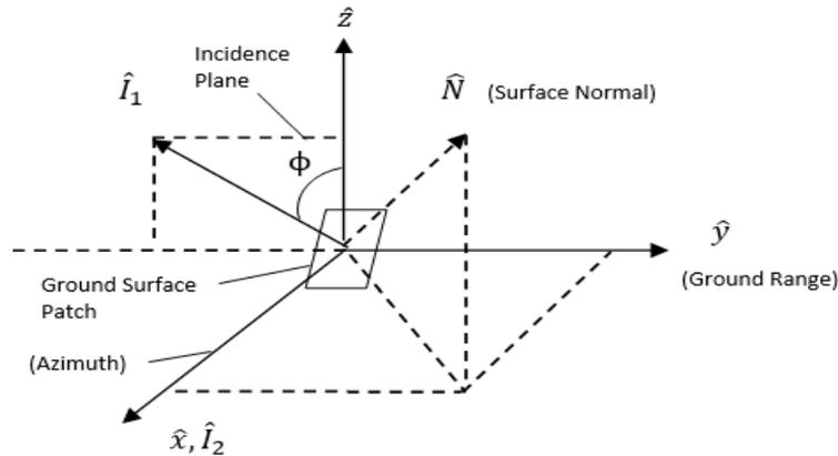
Figure 2.2 Diagram relates the orientation angle to the ground slope
