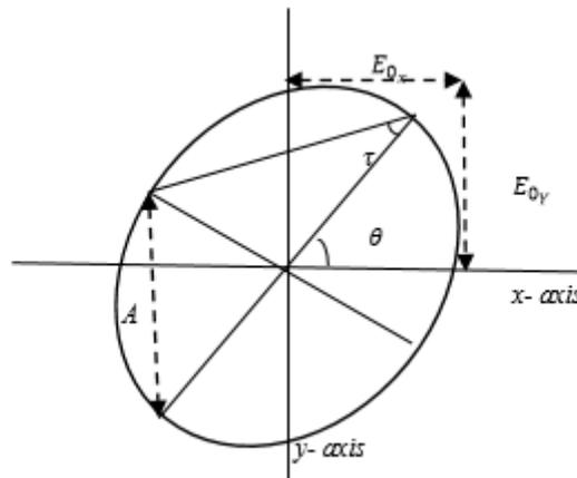
Figure 2.1 Graphical Representation of the Polarization Ellipse. ‘A’ is the amplitude of the ellipse,  $\theta$  is the orientation angle,  $\tau$  is the ellipse aperture.
