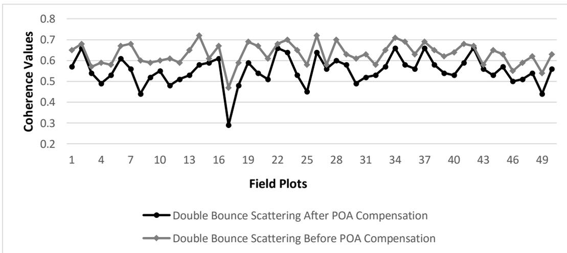
Figure 5.5 Coherence for the double bounce before and after POA compensation for 2013
