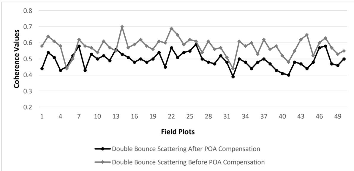
Figure 5.7 Coherence for the double bounce before and after POA compensation for 2014
