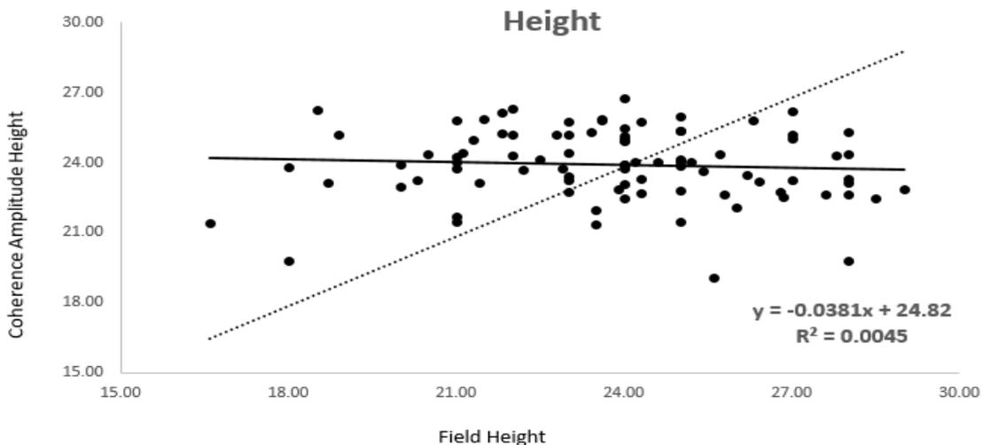
Figure 5.9 Scatter Plot between the Field height and CAI height before POA compensation for 2013
