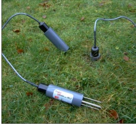
Figure 4-3 Theta probe soil moisture measurement
