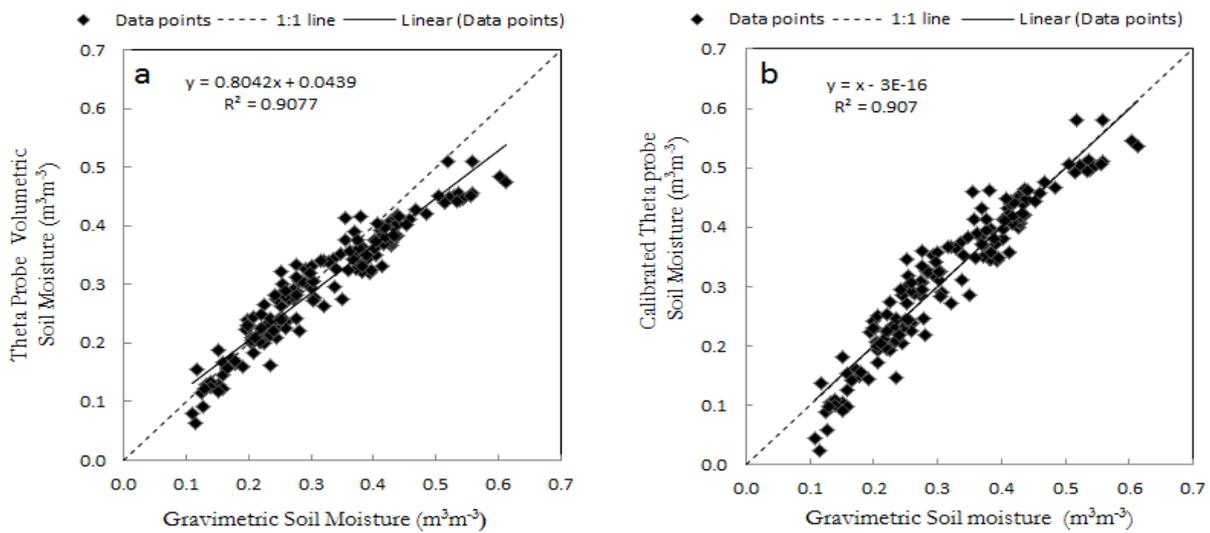
Figure 5-3 (a) Linearly related theta probe to gravimetric based volumetric soil moisture for the development of calibration equation; (b) calibrated theta probe versus gravimetric based volumetric soil moisture.
