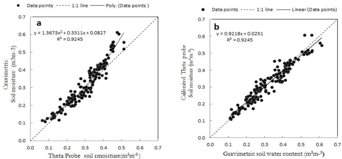
Figure 5-4 (a) Polynomial related theta probe to gravimetric based volumetric soil moisture for the development of calibration equation; (b) after calibrated theta probe using polynomial equation related to gravimetric based volumetric soil moisture with liner fit.
