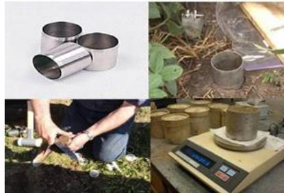
Figure 4-2 Gravimetric Sampling method
