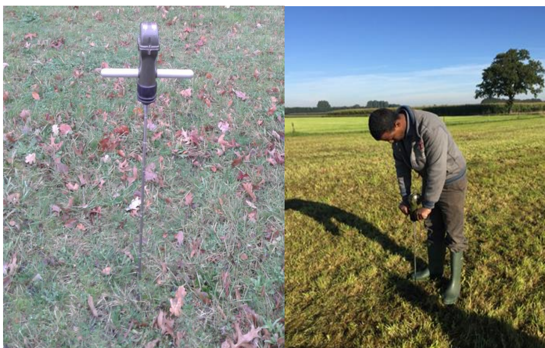
Figure 5: Picture shows cone penetrometer and field penetration resistance/cone index measurement.
