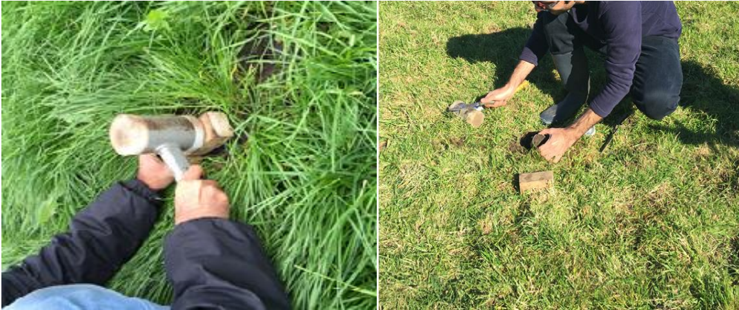
Figure 6: How Core soil sampled during field data collection, for gravimetric soil moisture estimation.
