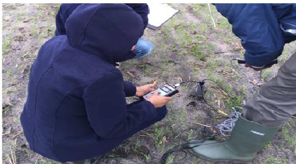
Figure 8: Photo shows Theta probe soil moisture reading during field data collection at SM_09.
