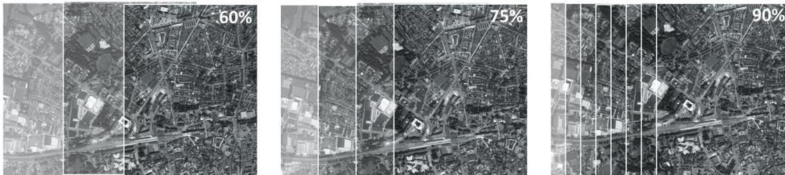
Figure 5. Sample of flight line with 60%, 75%, and 90% forward overlap
