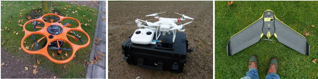
Figure 22. UAV employed on the research: Aibot X6 (left), DJI Phantom 2 Vision + (middle), and Ebee RTK (right)
