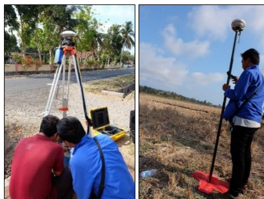
Figure 14: GNSS base and receiver for RTK in GCP measurement
