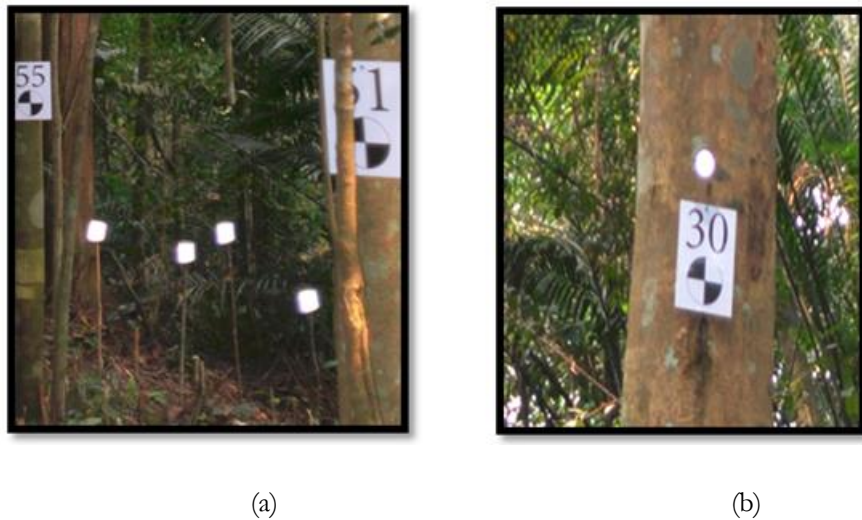
Figure 9: Cylindrical (a) and circular (b) reflectors from in the field
