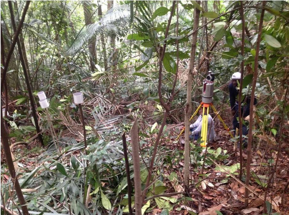
Figure 32: Dense undergrowth causing occlusions
