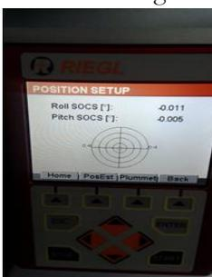
Figure 12: Levelled Terrestrial Laser Scanner
