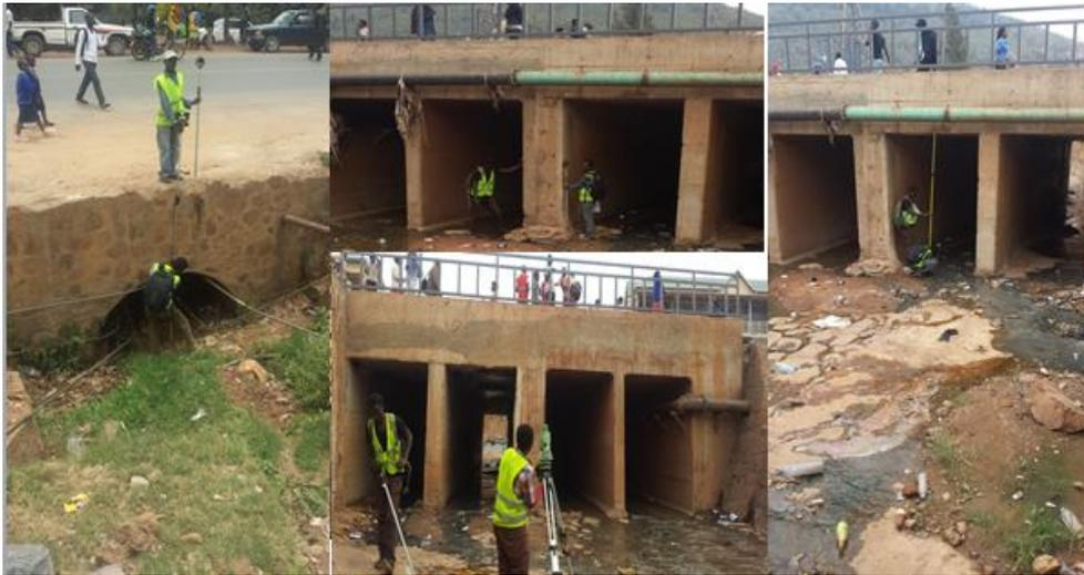
Figure 3.9: Sample photos taken while measuring location and cross-sections of culverts.
