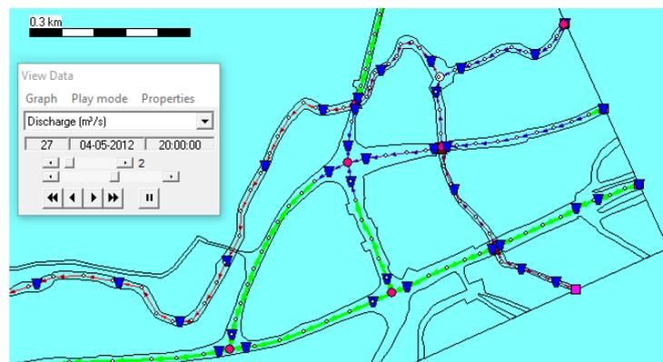
Figure 5.30: Snapshot of a zoomed-in road section during a combined 1D road and 1D river simulation.
