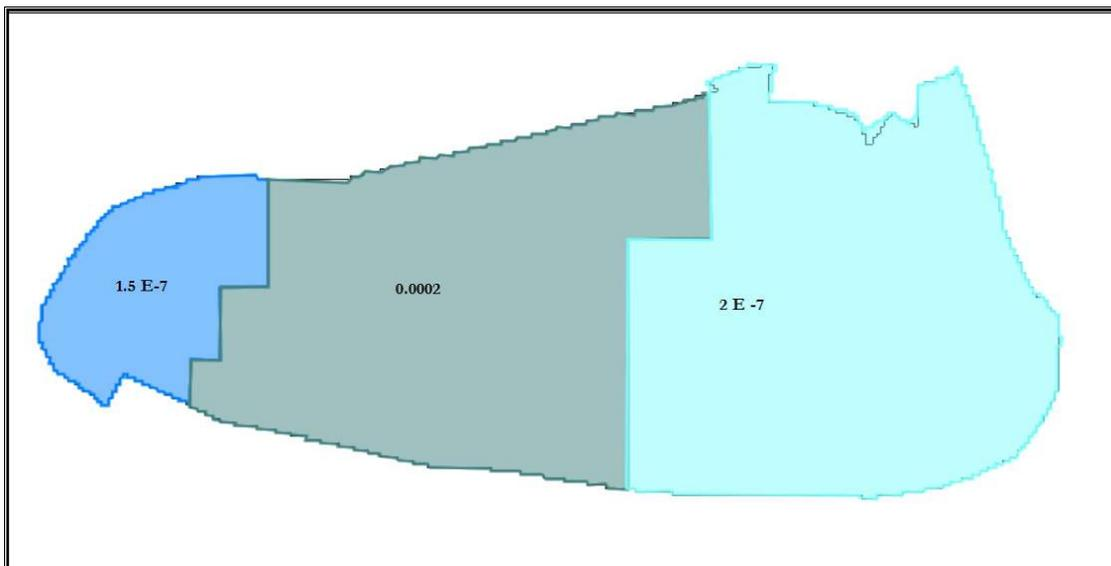
Figure 43: Vertical hydraulic conductivity (VKCB) in (m day<sup>-1</sup>) for M-K Mudstone aquitard.
