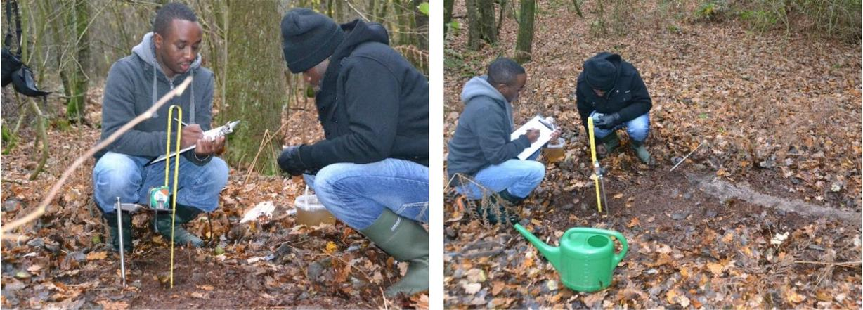
Figure 9: Fieldwork on inverse auger-hole method to determine saturated hydraulic conductivity. Left: the measuring apparatus used in the field. Right: the sandy soil core laid next to the bore-hole and time being taken by the Author (black jacket), whilst Mr. Sammy Njuki records the notes.
