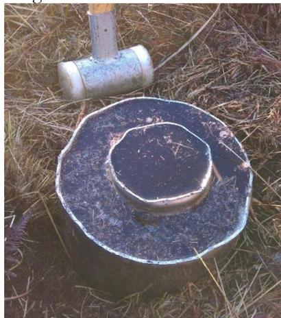
Figure 10: Use of the double rings infiltrometer to determine saturated hydraulic conductivity in the peat soils
