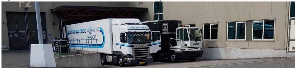
Figure 35 The terminal trailer at one of the two docks of the apple packing station.
