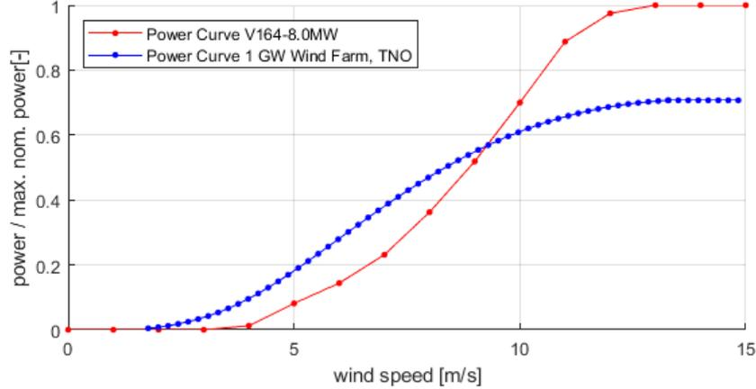
Figure 4.2: Power curves for the Vestas V164-8.0 MW turbine (red line) and a 1 GW wind farm (red line) with  $k=2.17$ .
