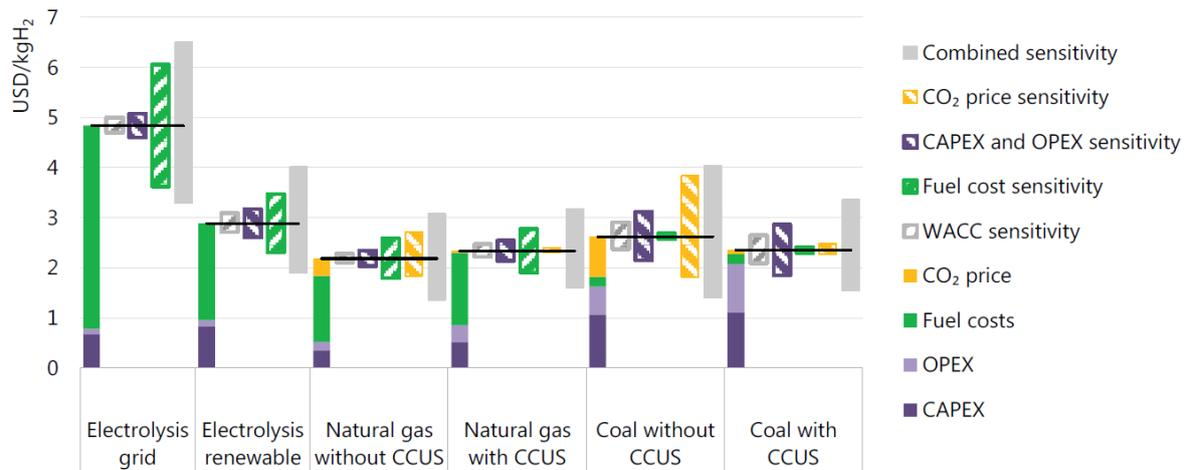
Figure 2.1: Hydrogen production costs for different technology options, 2030. Assumptions refer to Europe in 2030, reprinted from [12]
