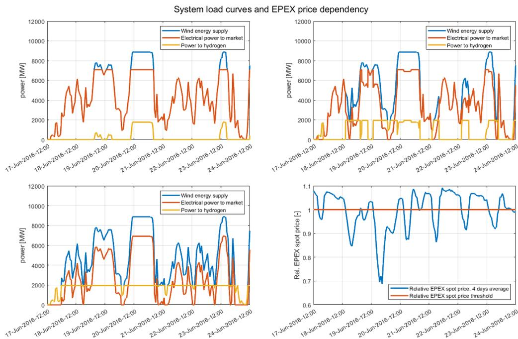
Figure 1: Load power for peak load operation mode (1) (top left), base load operation mode (2) (bottom left), market optimized operation mode (3) (top right) and the relative 4-day smoothed EPEX price (bottom) for a duration of 7 days
