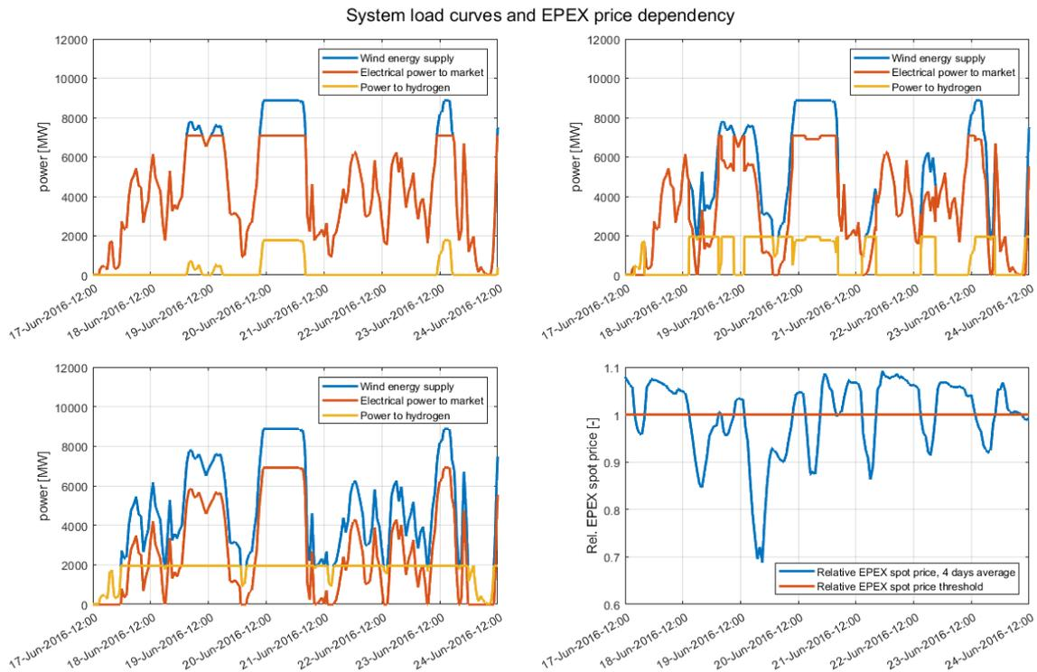
Figure 5.2: Load power of model functions for operation mode 1 (top left), operation mode 2 (bottom left), operation mode 3 (top right) and the relative 4-day smoothed EPEX price (bottom) for a duration of 7 days
