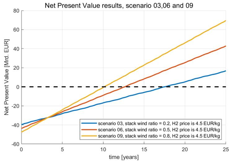
Figure 5.5: Net Present Value of the total system for scenario 03, 06 and 09, simulated over a period of 25 years.
