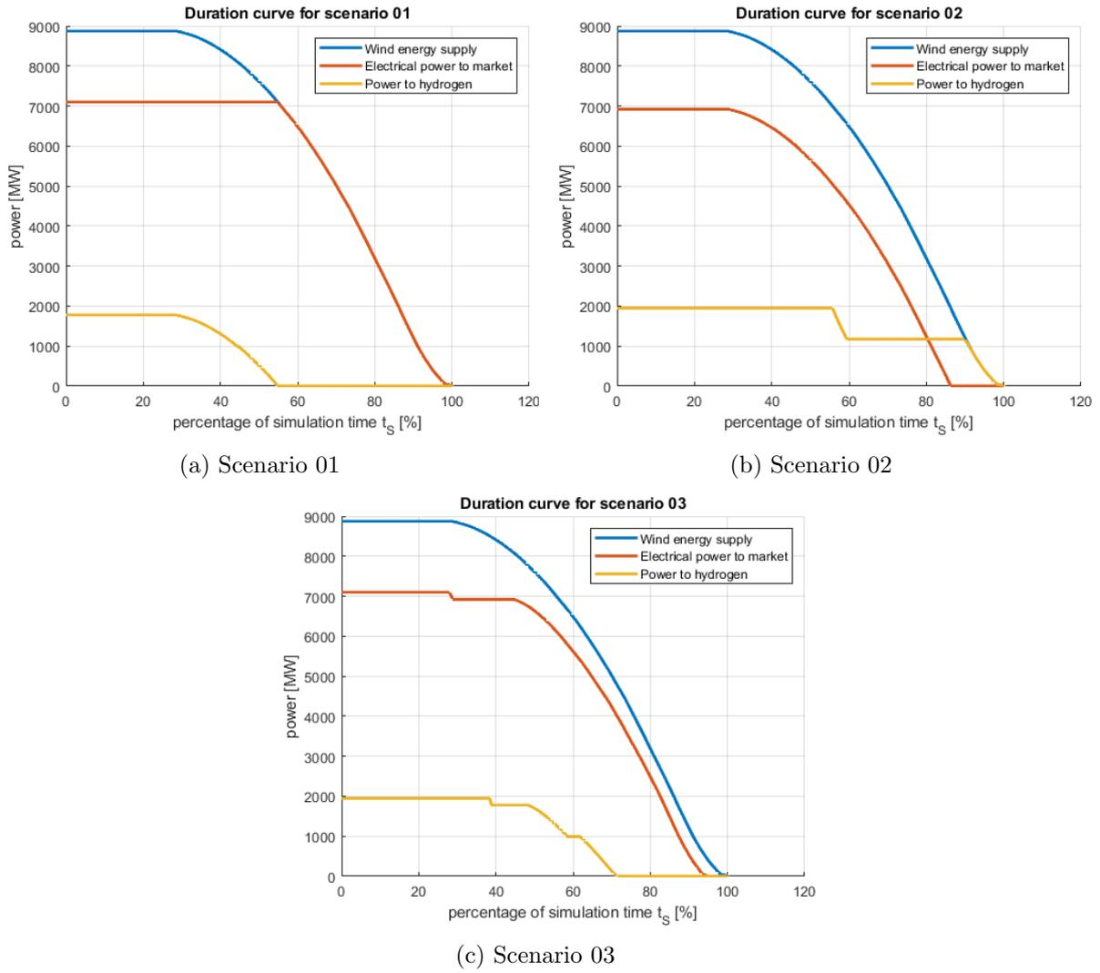
Figure 5.3: Load duration curves for simulation period 2013-2016
