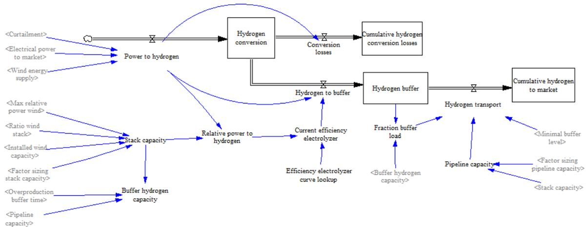
Figure 3.5: Schematic overview of the electrolyzer modeling including hydrogen buffer
