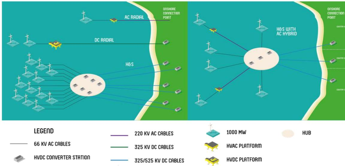
Figure 3.2: Grid connections systems including AC radial, DC radial and Hub & Spoke, reprinted from [7]
