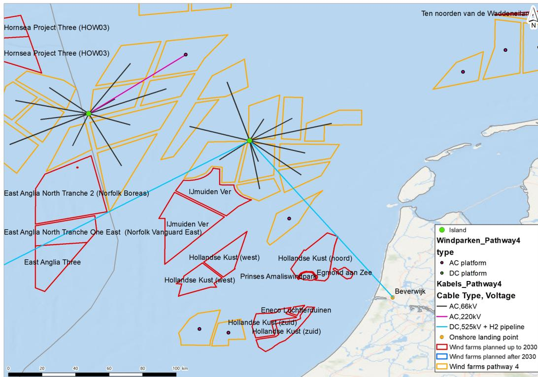
Figure 5.10: Extension of IJmuiden Ver (case 2): GIS Map for offshore wind farms up to 2030 (red) and new proposed wind farms (orange) in the North Sea. Reconstructed from the GIS model created and owned by Witteveen+Bos for the NSWPH project.
