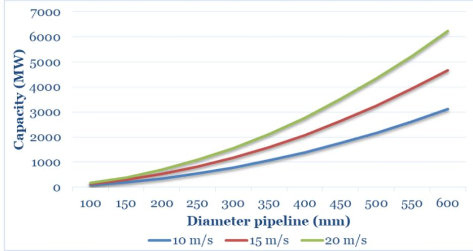
Figure 3.7: Power of gas pipeline vs diameter, reprinted from [34]
