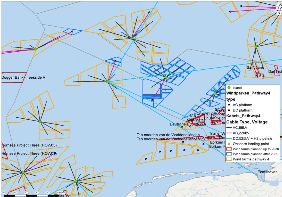
Figure 5.9: Around Centrale Oestergronden (case 1): GIS Map for offshore wind farms up to 2030 (red), planned after 2030 (blue) and new proposed wind farms (orange) in the North Sea. Reconstructed from the GIS model created and owned by Witteveen+Bos for the NSWPH project.
