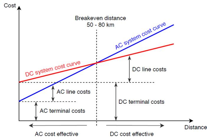
Figure 3.1: AC and DC system costs based on transmission distances, reprinted from [20]
