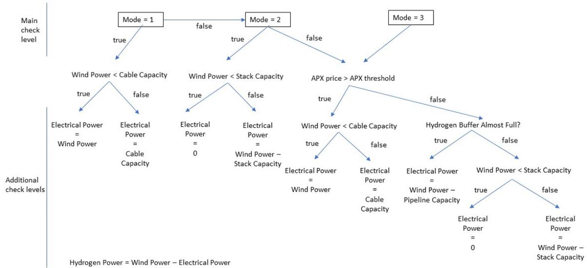
Figure 4.3: Schematic flow chart of model framework for operation mode 1,2 and 3.
