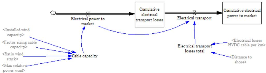
Figure 3.8: Schematic overview of the model for electricity submission
