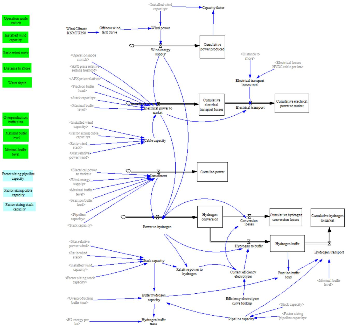
Figure B.1: Technical model as created in Vensim energy simulation software
