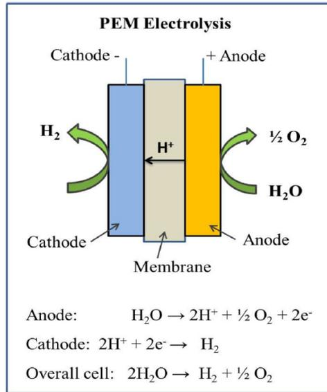
Figure 1.1: Schematic overview of PEM water electrolysis, reprinted from [9]
