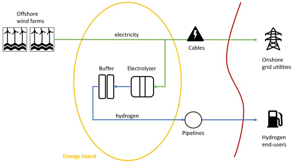
Figure 1.2: Overview of the energy hub concept including hydrogen production
