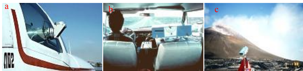
Figure 2.2. Cospec from the plane (a), from the vehicle (b) and from a stationary tripod (c).
