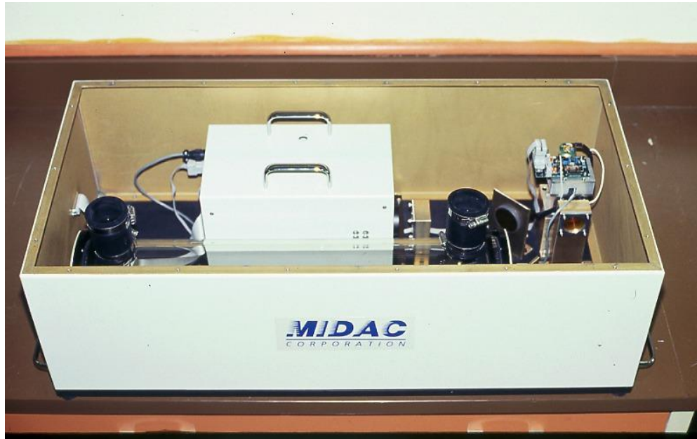
Figure 2.3. Interior view of a closed-path FTIR. It shows gas cell, Michelson interferometer, globar light source, helium-neon laser, and MCT detector.
