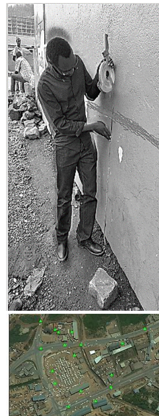
Figure 3.7: Marking water level on walls of building and its spatial locations during fieldwork
