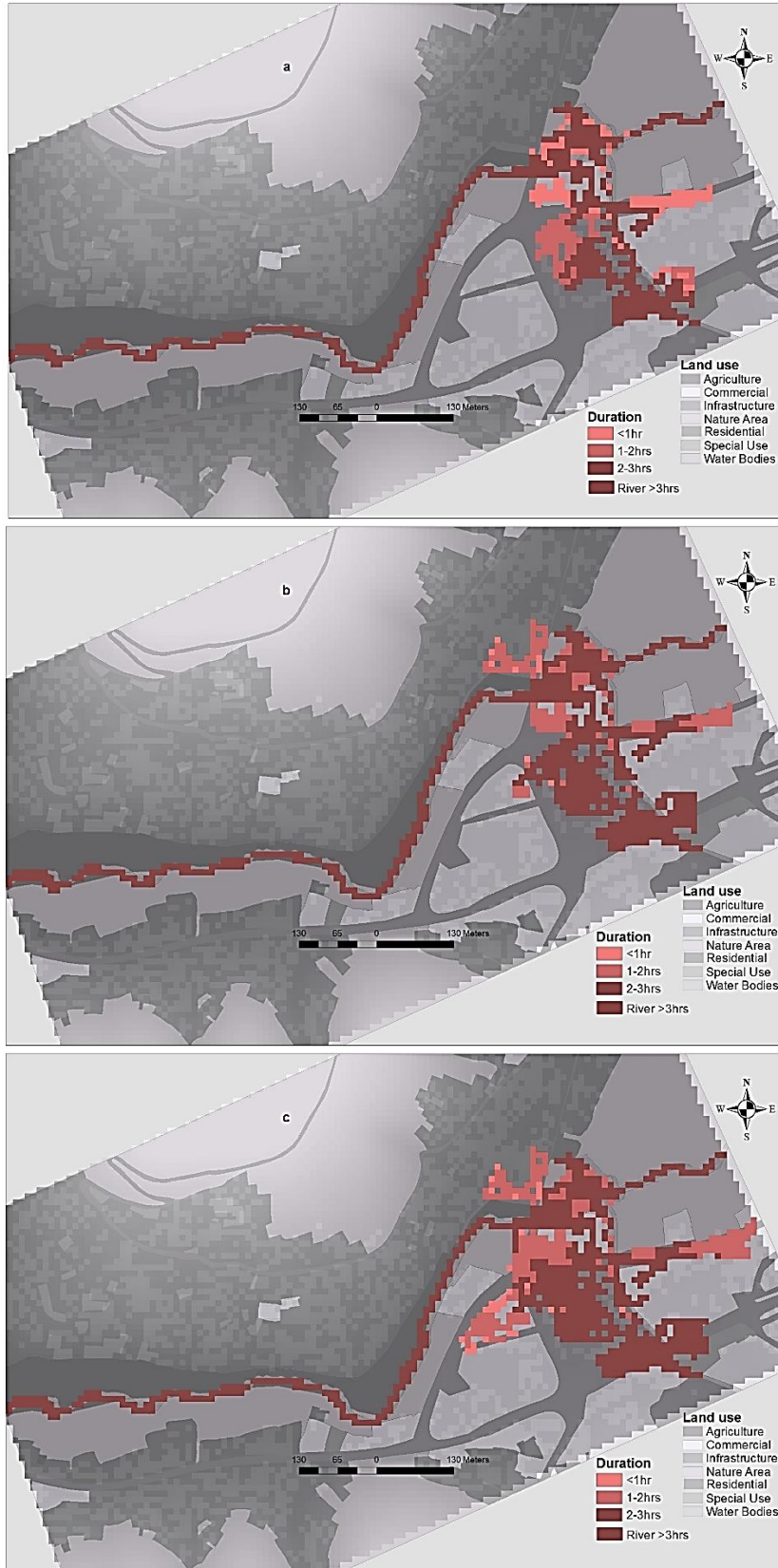
Figure 5.8: Spatial distribution of estimated duration of flash floods in hrs for different return periods (a) 10 year return period (b) 20 year return period (c) 50 year return period.
