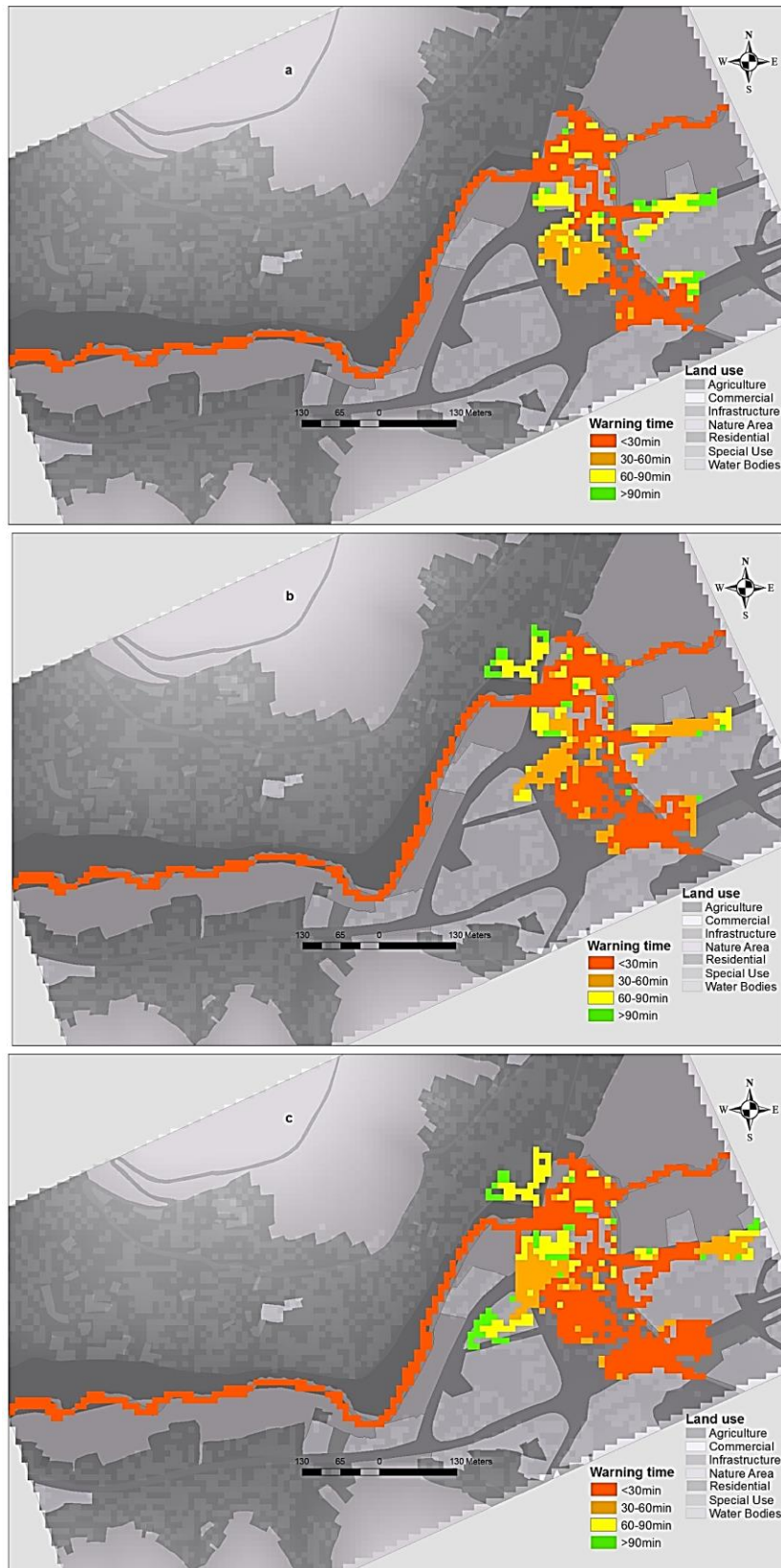
Figure 5.7: The spatial distribution of the arrival time of the first flood water (Warning time) with event of different return period of (a) 10 year return period (b) 20 year return period (c) 50 year return period.
