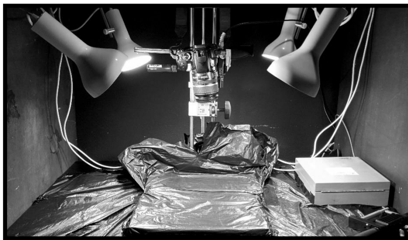
a) ASD 8° optical fibre set-up
