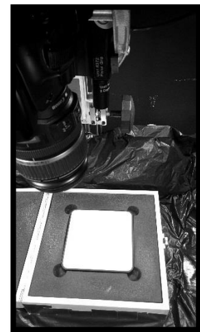
b) White reference plate with view of 8° optical scope
