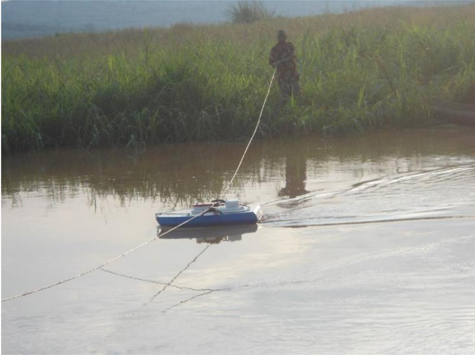
Flow measurement using an ADCP device.
