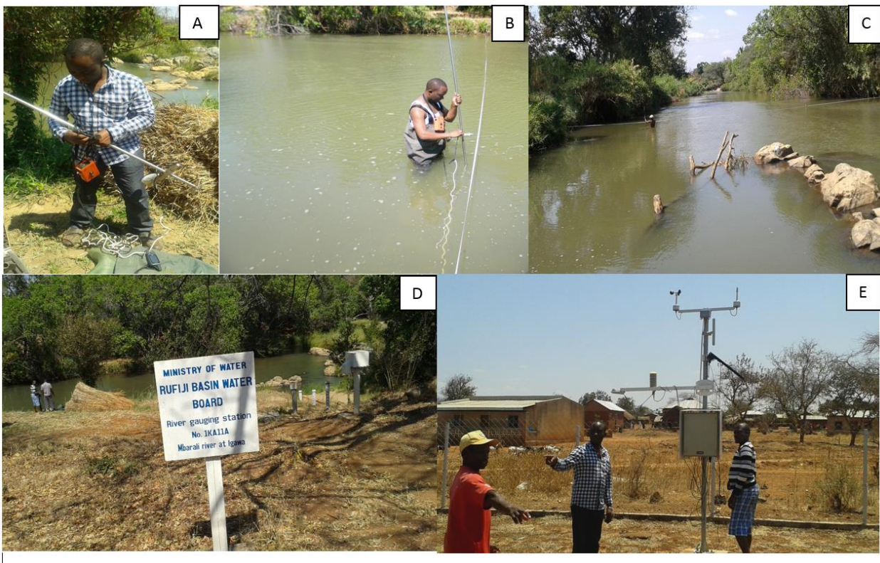
Figure 7: Picture of different activities undertaken during field trip to Mbarali sub-catchment. A= Configuration of current meter which is used to take discharge measurements, B= Taking discharge measurement at Mbarali river at Igawa (1AKA11A), C= Mbarali river at Igawa section, D= River gauging station automatic and manual instruments and E= Igawa meteorological station.
