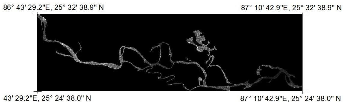
Figure 4.3 River extracted from RISAT-I image dated 04 Aug 2013 for evaluation of water bodies.
