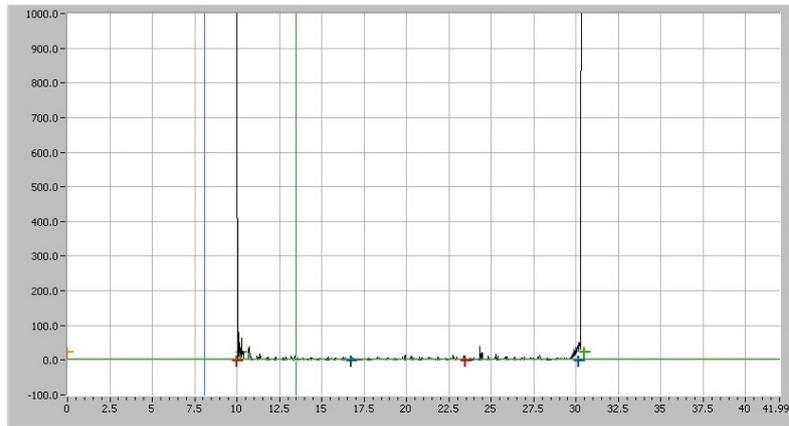
Figure 2.1: Receiving current with no residual current (ProRail, 2020)
