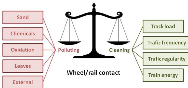
Figure 2.3: Factors influencing wheel/rail contact (Wybo, 2018)
