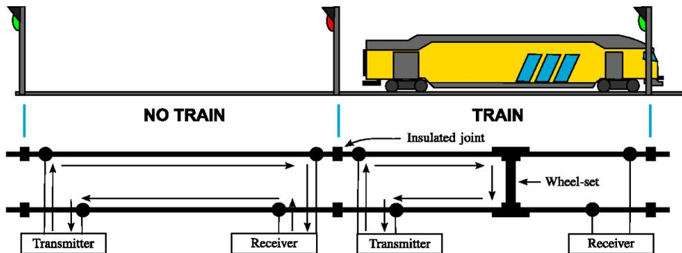
Figure 1.2: Track circuit (Bruin et al., 2016)
