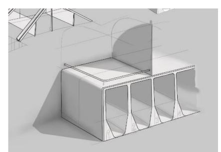
This is a sample of one of the different concepts which were worked out in the ideation process. This example shows storage boxes which will house the bicycles to be stored. On top of the boxes a luggage shelf is installed to improve the overall footprint by removing the need for dedicated luggage shelves. This concept was ultimately not chosen, but represents the different approaches taken to solve the problem.
