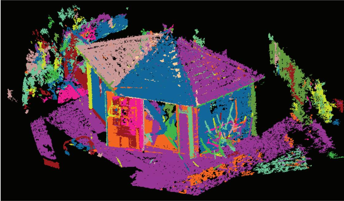
Figure 4.3: Point cloud after segmentation.
