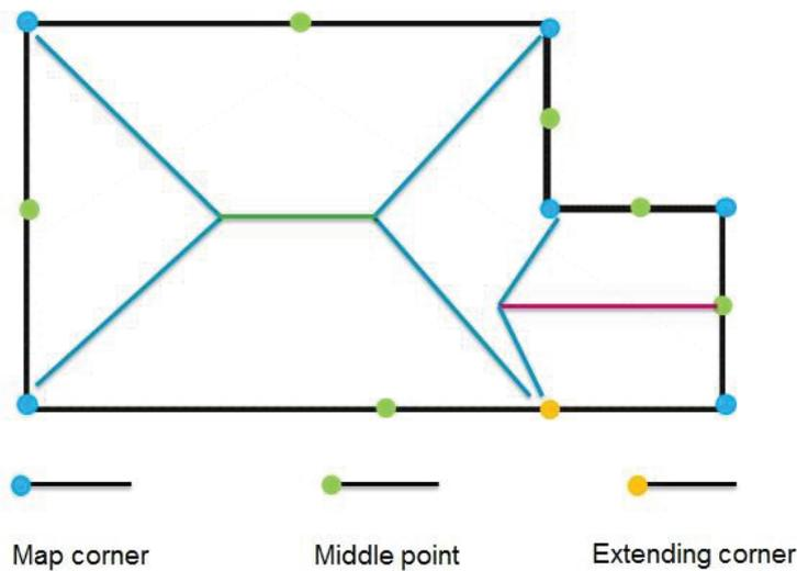
Figure 3-9 Three types of candidate corners with initial roof skeleton
