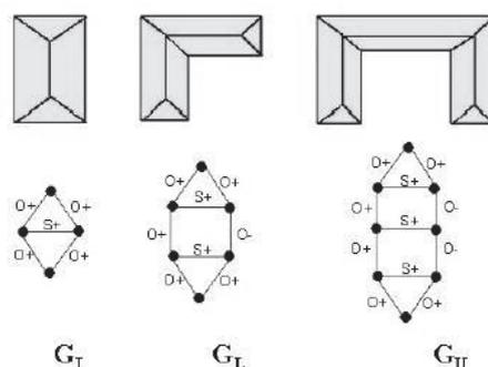
Figure 2-2 Roof topology graphs with corresponding simple parametric shapes(Verma et al., 2006)
