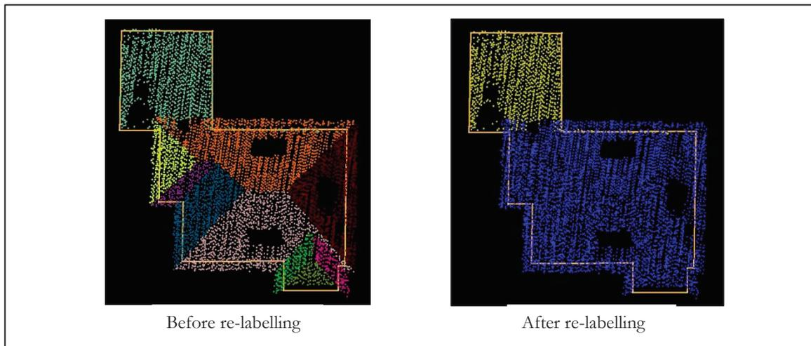
Figure 3-6 Laser points re-labelling
