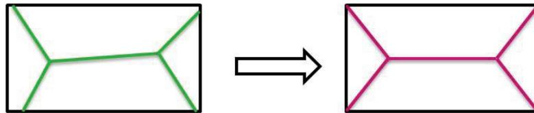
Figure 3-11 Expected result of roof skeleton optimization in a simple hip roof
