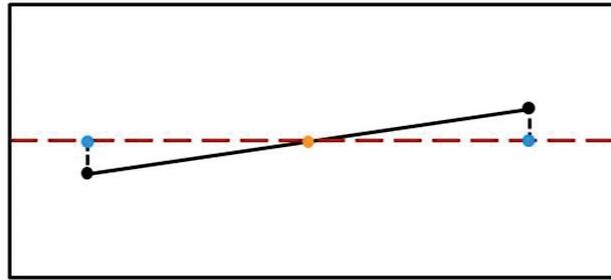
Figure 3-10 Original internal points (black) are adjusted to fit building orientation (dark red dash line).
