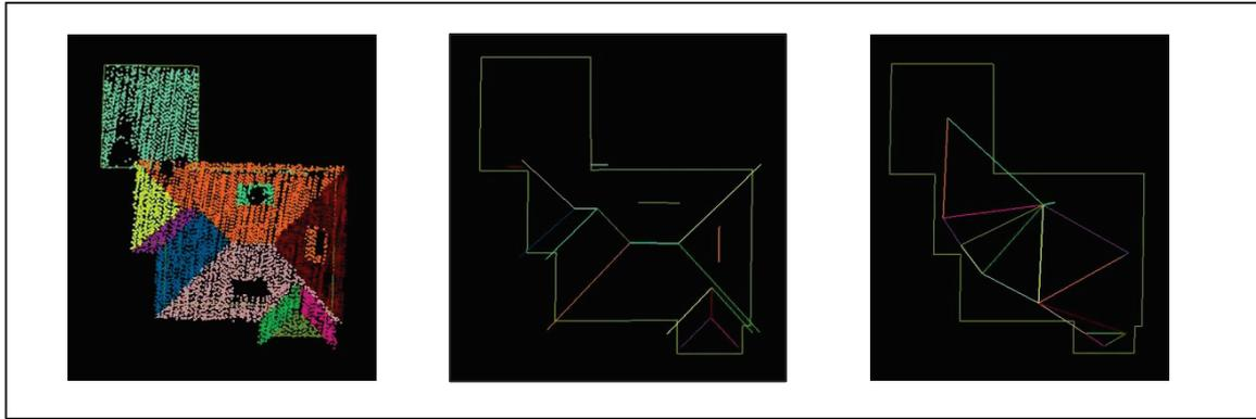
Figure 3-2 Roof segments (left), structure lines (middle) and roof topology graph (right)
