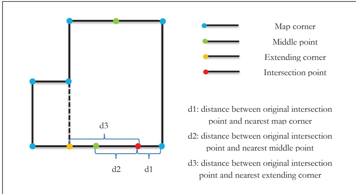
Figure 4-6 Three distances of one intersection point
