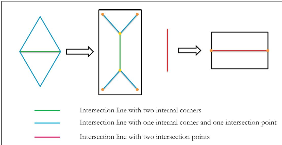
Figure 3-4 Three types of intersection lines
