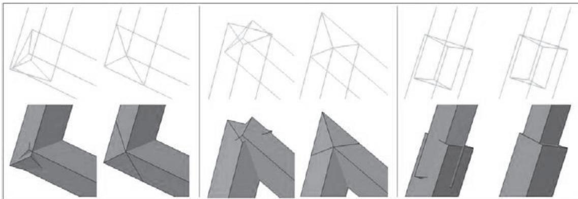
Figure 1-2: Mismatching problem when merging adjacent primitives(Huang et al., 2013)
