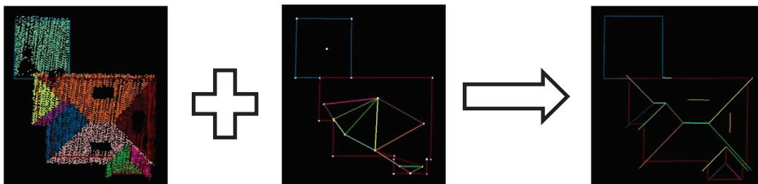
Figure 3-8 Initial roof skeleton creation from laser points and topology graph
