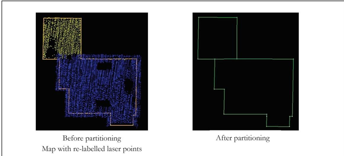
Figure 3-7 Map partitioning by re-labelled laser points
