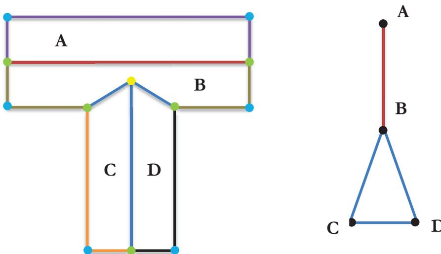
Figure 3-12 Roof faces detection from topology graph and building outlines
