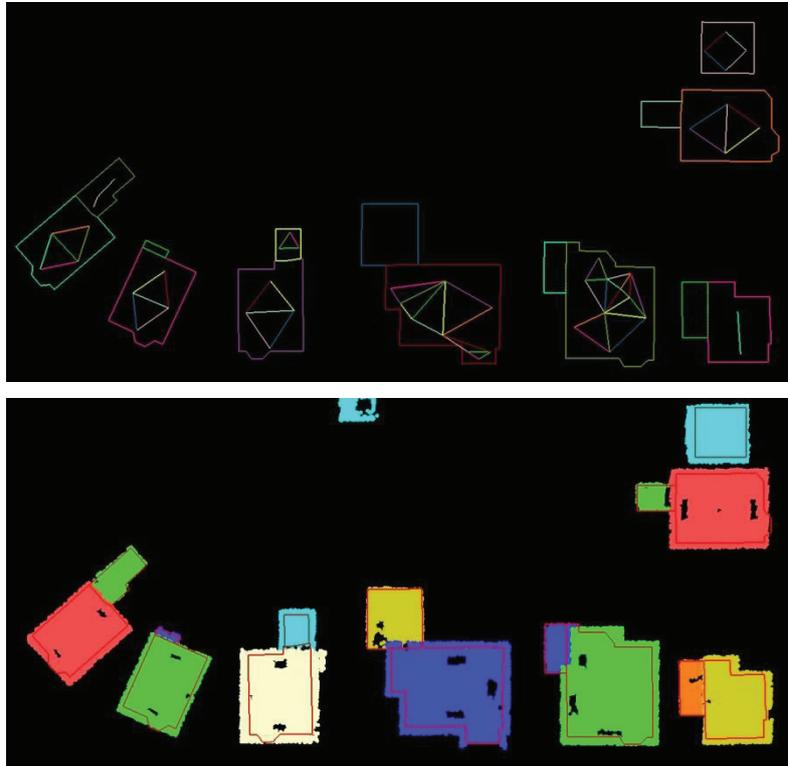
Figure 4-3 Partitioned map data with related partitioned topology graph (top) and Partitioned map data with re-labelled laser segments (bottom)
