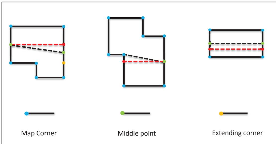
Figure 4-5 False intersection lines assignment
