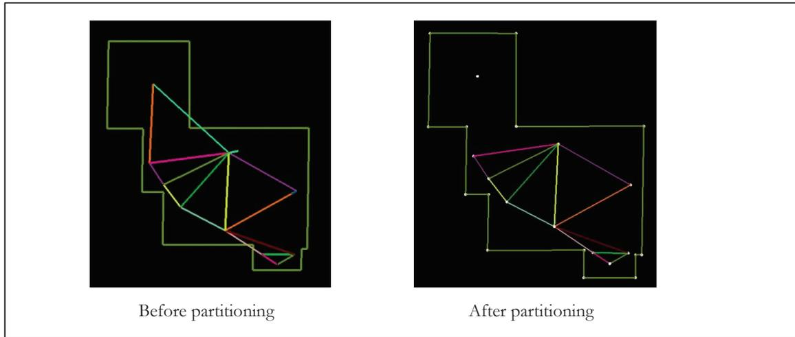
Figure 3-5 Roof topology graph partitioning
