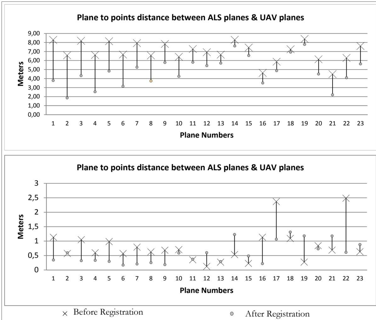
Figure 4.13: Impact of Vertical Shift application on residuals (mean) of Distance (above) shift not applied (below) shift applied
