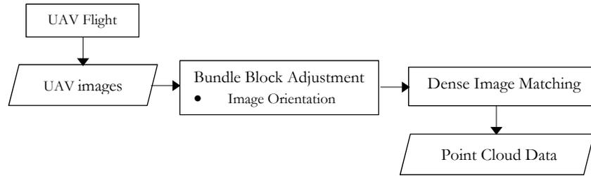
Figure 2.2: Point cloud generation process using UAV images
