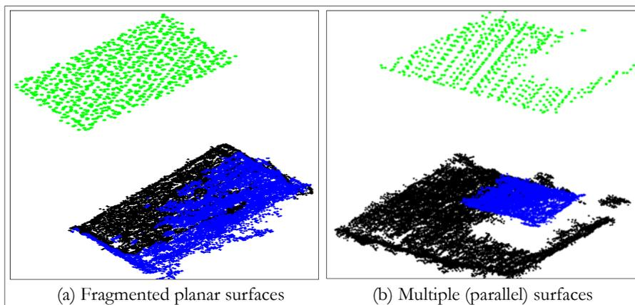
Figure 3.8: Selection of fragmented and multiple planar surfaces using 1: n approach
