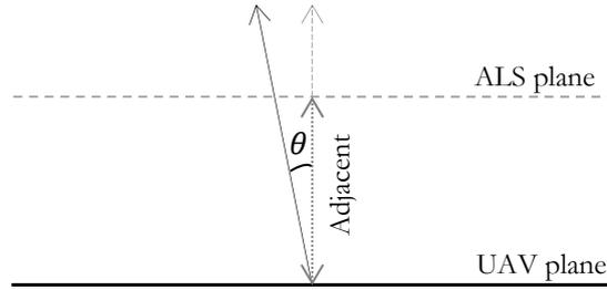
Figure 4.11: Estimation of threshold value for normal angle deviation
