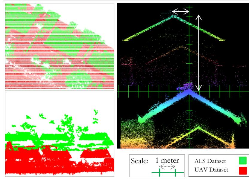
Figure 1.2: Illustration of horizontal & vertical shift found in both datasets
