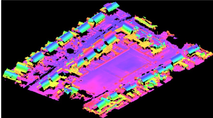
Figure 4.2: Generated Point Cloud through UAV images and visualized in PCM
