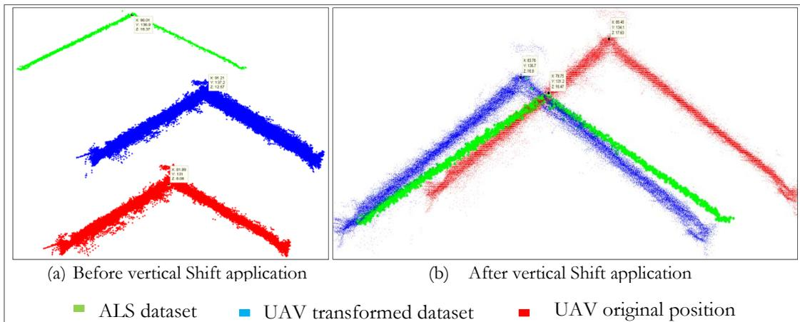
Figure 4.12: Effect of vertical shift applied on UAV dataset
