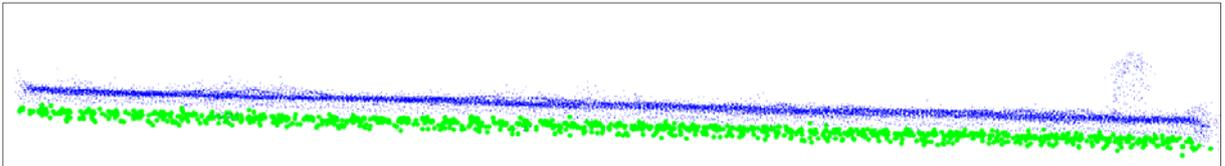
Figure 5.1: ALS (green) plane with UAV (blue) plane (ground control points used)
