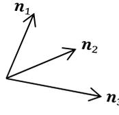
Terms  $\mathbf{n}_1$ ,  $\mathbf{n}_2$  and  $\mathbf{n}_3$  are normal vectors of three planes. This value should be significantly non-zero and it would be better to set a threshold value for determinant value to keep only reliable non-parallel combinations. It will automatically discard those weak combinations whose determinant
