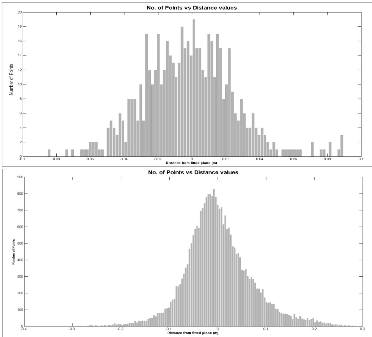
Figure 4.3: Comparison of Planar accuracy with signed distance values (above) ALS (below) UAV
