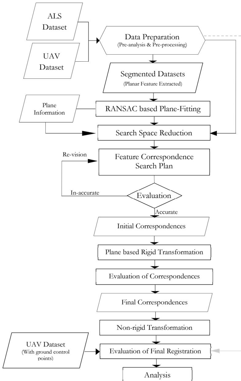
Figure 3.1: General Process of Feature based Registration between ALS and UAV datasets
