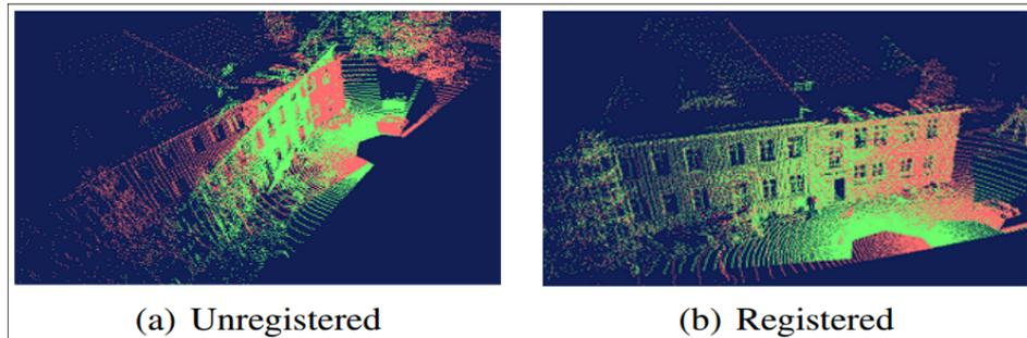
Figure 2.3: Result of registration using planar surfaces (Dold & Brenner, 2006)
