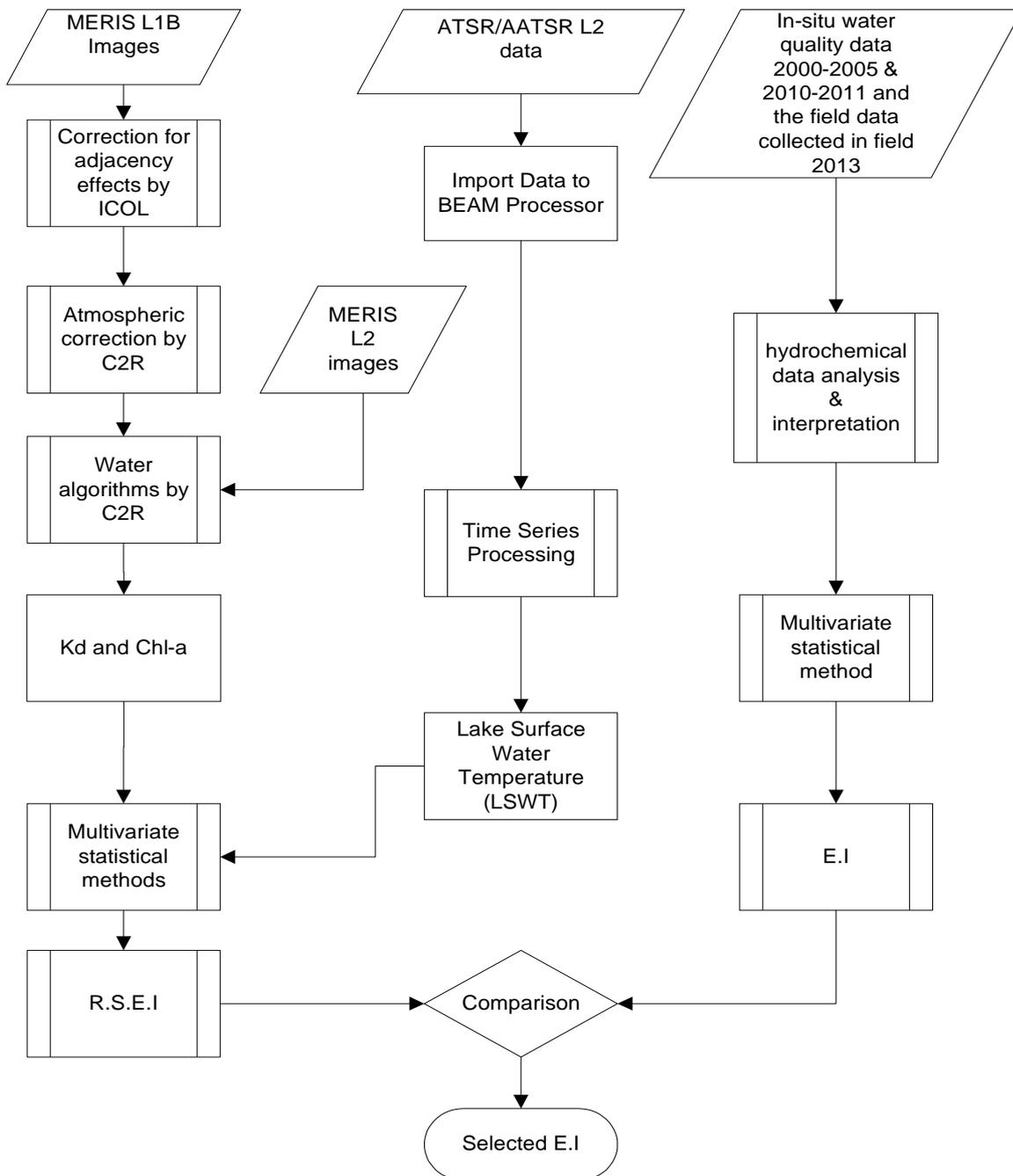
Figure 4.3: The schematic procedures for pre-processing, processing and derivation of Chl-a, Kd, and E.I
