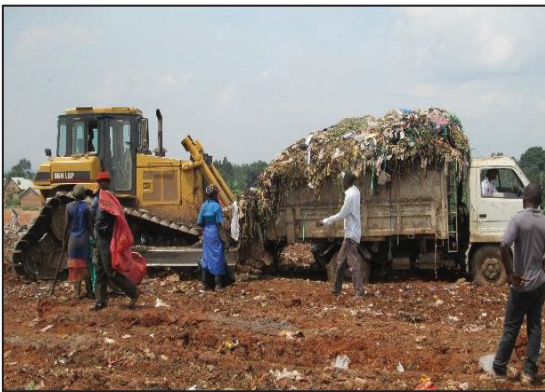
Figure 21. Stuck truck being pushed by a dozer
