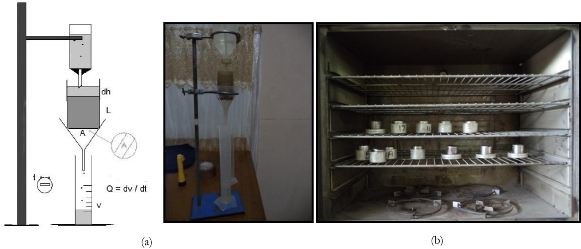
Figure 3-17 (a) Pseudeu laboratory method used Ksat Measurement (Alkema, 2009) and field observation and (b) Heating soil samples in oven for 24 hours to measure the porosity values
