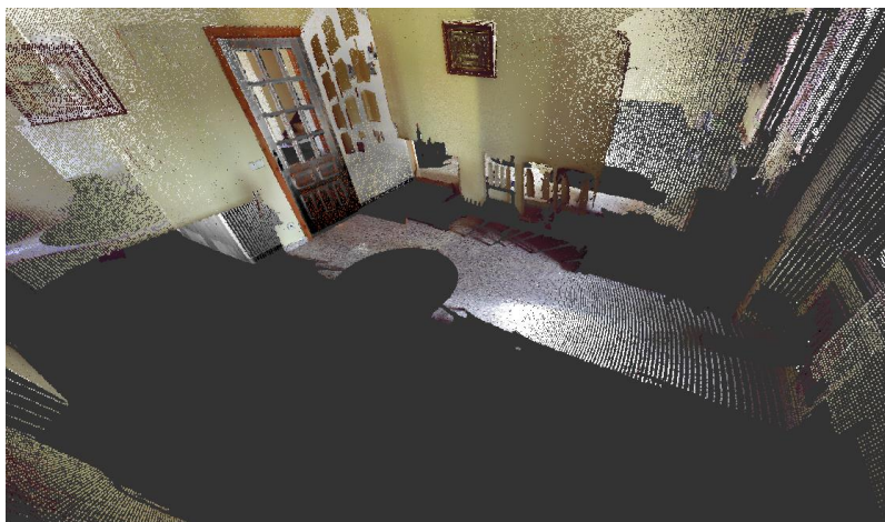
Figure 5-4 The occlusion of the point cloud data
