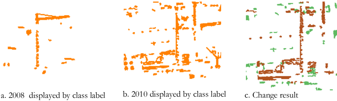
Figure 4-15: Example of false negatives, in (c) brown colour represent changed components and green colour unchanged components
