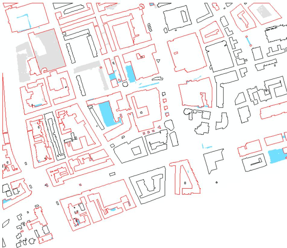
Figure 5-14: Building polygons earmarked for updating (red) and those that are unchanged (black). The relevant changes are shown in the two classes of building extension (blue) and mixed objects (grey).
