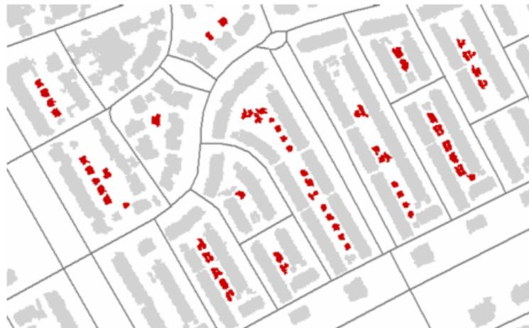
Figure 2-8: Segments falsely marked as new buildings (red) which were in fact omitted in the map due to mapping rules. Source: Vosselman et al., (2004).
