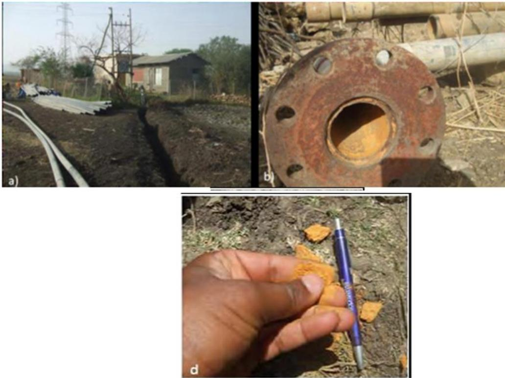
Figure: a, PVC Pipes to replace damaged metallic pipes due to corrosion (salinity) problem and d, metallic pipe change to soil due to corrosion problem (Berhane et al., 2013)
