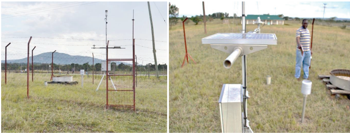
Figure 4: Weather station at the Mara River Water Users Association (MRWUA) office in Mulot. The station has a tipping bucket and a manual rain gauge. The weather station automatic measuring instruments are not yet connected to the data logger. Picture by Vekerdy Z. (2013)
