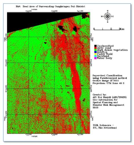
Figure 5-30. Supervised classification of surrounding areas of dirt road using parallelepiped method.
