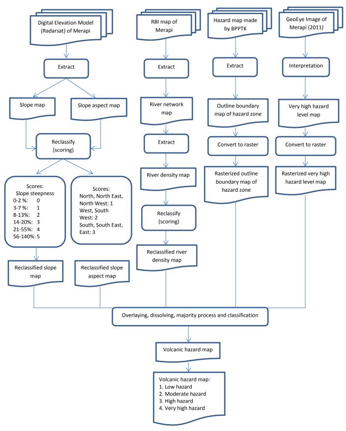
Figure 4-7. Flowchart of detailed volcanic hazard mapping
