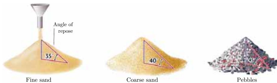
FIGURE 3.6: Typical angles of repose as for granular materials of different size. Note that angularity is not taken into account in this figure. [Modified after Grotzinger & Jordan (2010) 59 ]
