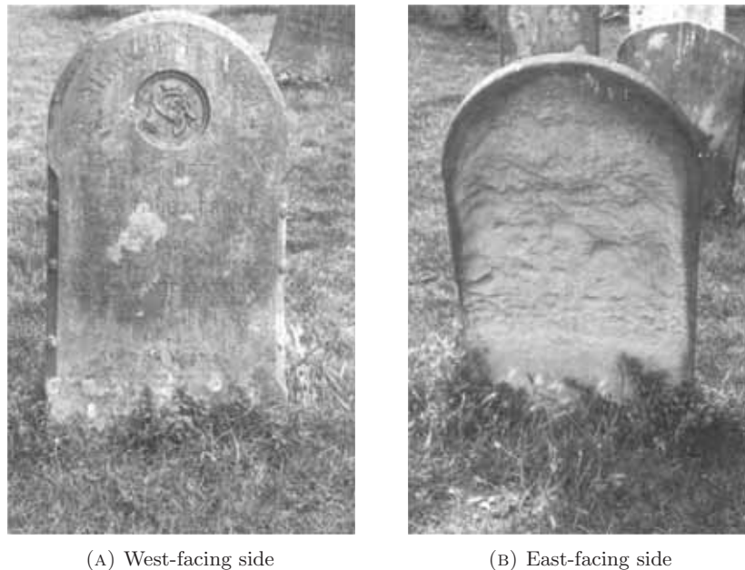
FIGURE 2.8: The (A) slightly weathered and (B) severely weathered side of a sandstone tombstone dated 1883. The difference is due to the prevailing western winds in the region. [Wymondham Abbey (U.K.), Price (1995) 77 ]
