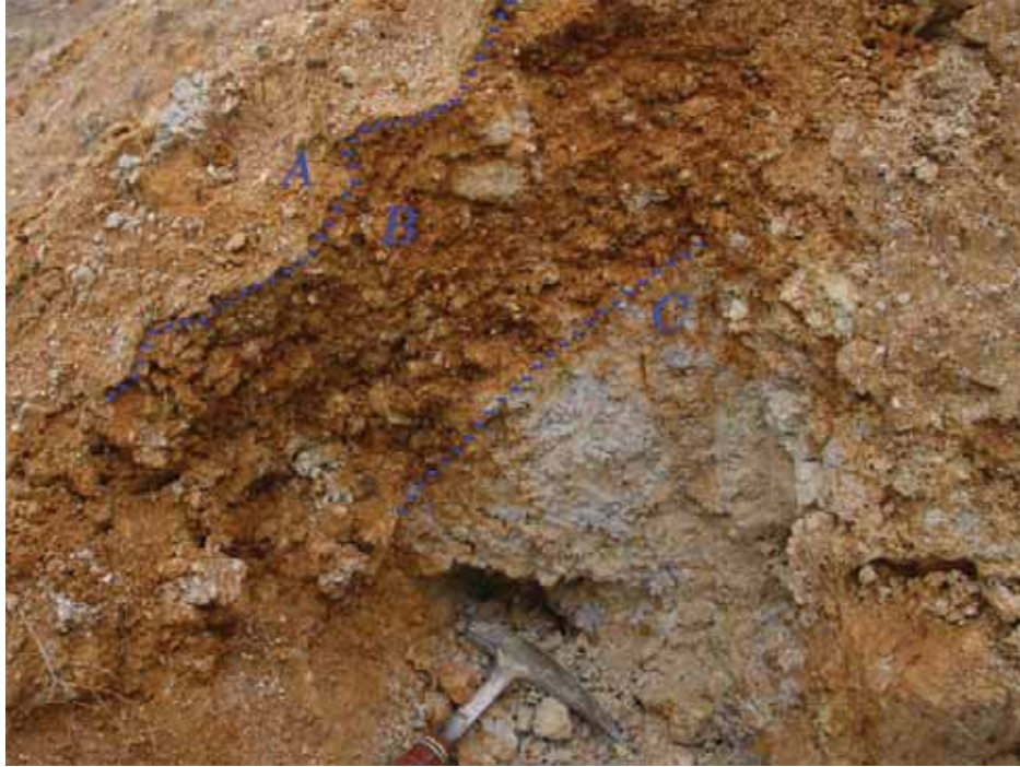
FIGURE A.2: Weathering profile at the northwestern part of Ostrelj overburden waste dump. A: Orange crust; B: 22 cm thick orange layer of sandy clay; C: Grey in-situ residual soil in a matrix of yellow clay. [10th November 2011, Bor, Serbia (44°5'6.43" N; 22°6'0.6317" E)]
