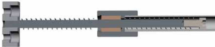
(A) Digitally drawn cross section of the spring-tipped rod.
