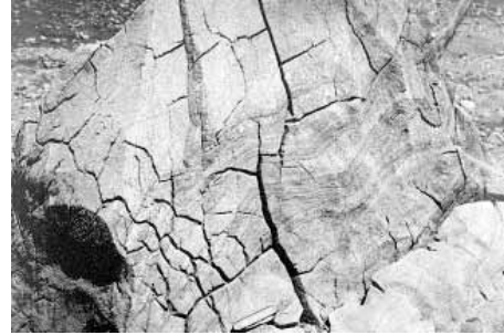
(B) Thermal fatigue of a rock (Andes, Argentina). Notice that the fractures do not follow the planes of weakness, i.e., discontinuities. [K. Hall 71 ]
