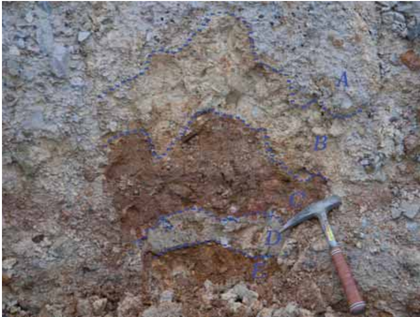
FIGURE A.1: Weathering profile at the northwestern part of Ostrelj overburden waste dump. A: Grey crust; B: \pm 15 cm thick yellow layer of completely weathered residual clay; C: \pm 15 –20 cm thick red sandy clay layer; D: 8 cm thick grey residual clay with some red spots; E: Orange sandy clay. [7th November 2011, Bor, Serbia (44°5'16.2" N; 22°6'37" E)]
