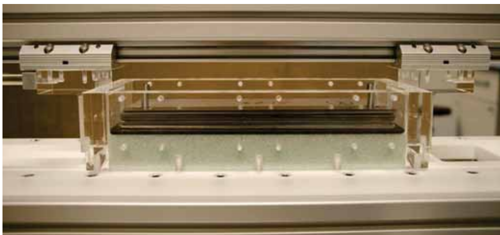
FIGURE 5.2: Close-up of the upper-container while it is loaded with a sample. The normal stress is applied by stainless steel plates that are on top of a holder (black PVC) that tightly fits the upper container.
