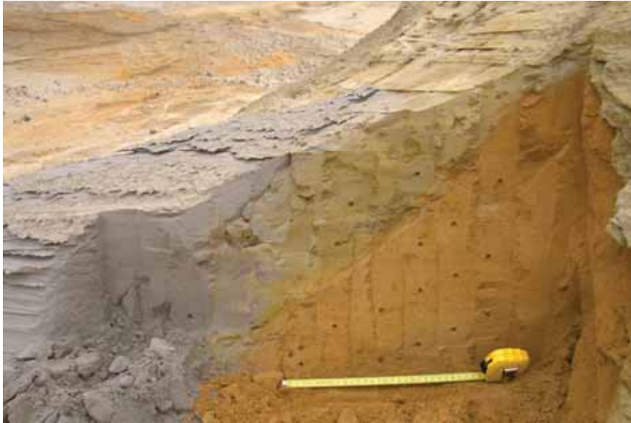
(A) Discolouration of tailings material. [3rd November 2011 (44°5'12.2" N; 22°9'34.7" E)]
