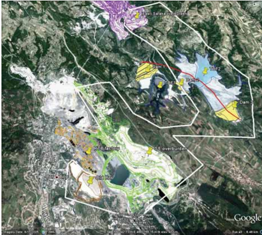
FIGURE 3.8: Satellite view of Bor indicating Old Bor TDF (brown), Ostrelj overburden (green), Krivelj TDFs 1&2 (blue) incl. three tailings dams (yellow), Saraka overburden (purple), RTB factory (orange), Kollektor (red), project area border (white). The North arrow is pointing straight up (poorly visible in the top right corner of the image). [Satellite imagery: Google™Earth 2005]
