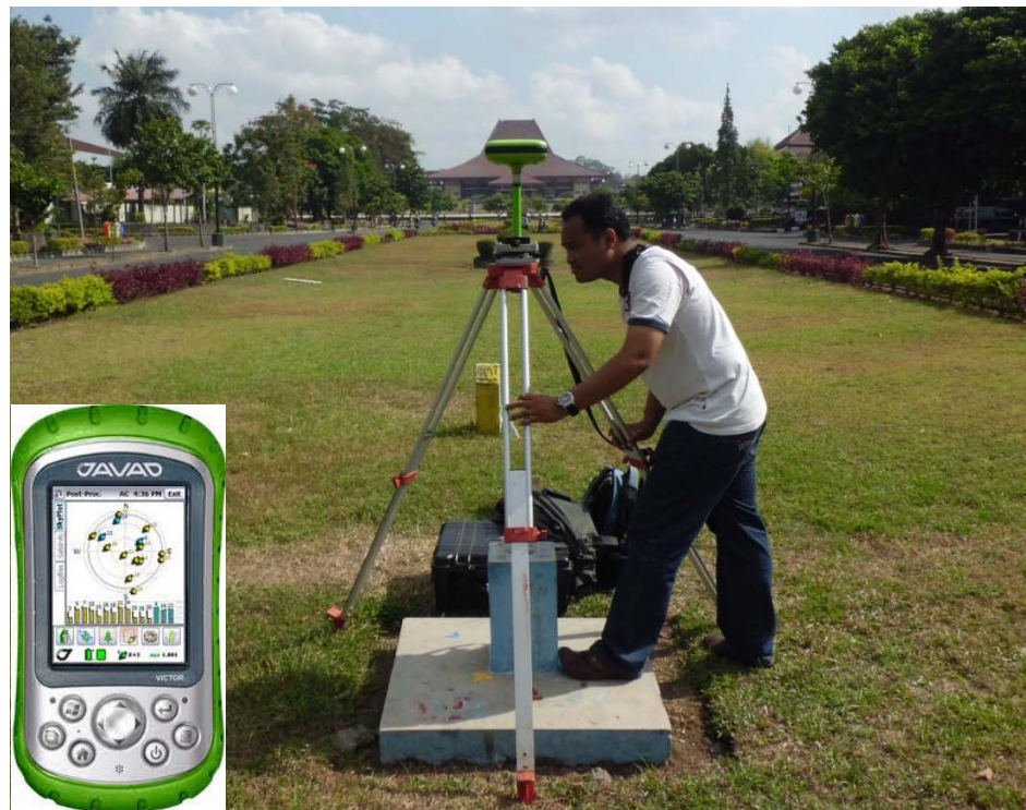
Figure 6.1 Base station BM number N005 and Javad Triumph L1/L2 Geodetic GPS source fieldwork 2012
