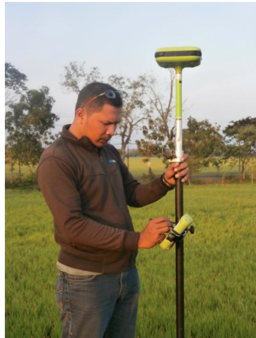
Figure 3.8. RTK method for detailed spot height measurement
