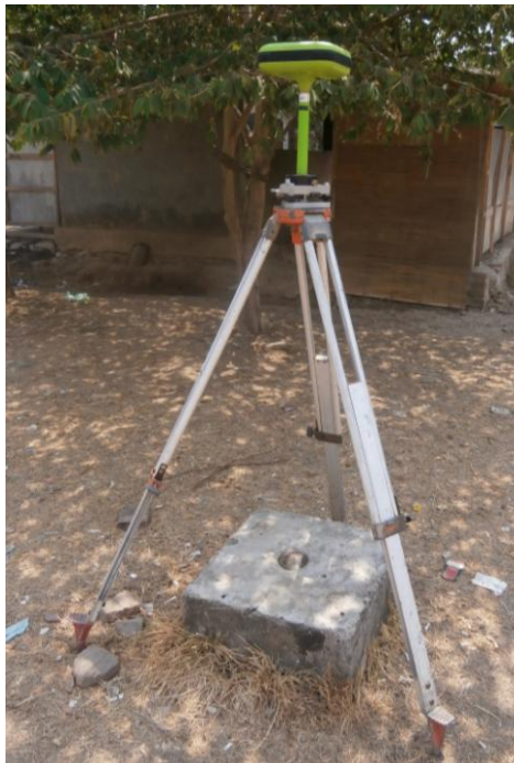
Figure 3.7. Static DGPS for base point measurement
