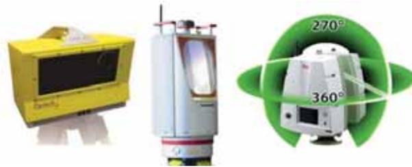
**Figure 4:** Types of TLS instruments: Optech ILRIS 3D, window-like scan system (left); RIEGL VZ-6000, panoramic with a polygonal wheel (centre); Leica ScanStation C10, with a Palmer scan system (right).
