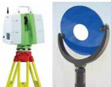
**Figure 11:** Leica ScanStation C10 (left) and Leica HDS (6' circular tilt and turn) target (right), mounted on tripods.
