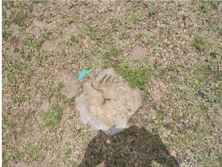
Figure 1: A survey beacon private land plots after sub-division found within conservancies
