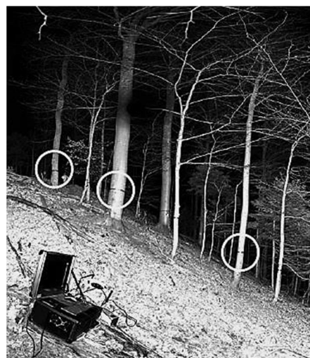
Figure 36. Intensity image of a part of the sample plot. Reflecting tapes marks a height of 1.30 above ground (Thies et al., 2004)
