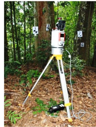
Figure 12. Setting TLS on a tripod
