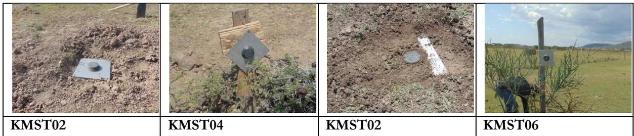
Figure 18: Examples of antenna setups improvised to increase the reception with the telecommunication network for the remote exchange of data.
