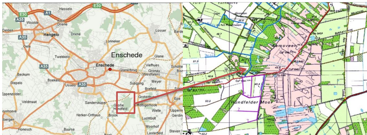
Figure 1.3 The whole area of Aamsveen. The red line is the old channel with the tube, the tube followed the border from the purple line; the purple lines show the old system at the area where the canal was later installed and the blue lines show the new canal channel dug in 2011.
